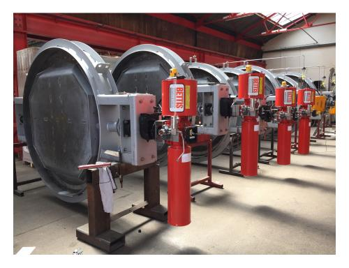
These range of dampers are specially engineered for applications involving process gases containing SO<sub>2</sub> / SO<sub>3</sub> which are butterfly or louvre dampers designed to suit any duct size(typically Ø<sub>3</sub>00mm – Ø<sub>3</sub>000mm). With SS<sub>3</sub>04H construction they are resistant to corrosion, high temperature (up to 800 Deg C), and creep.
