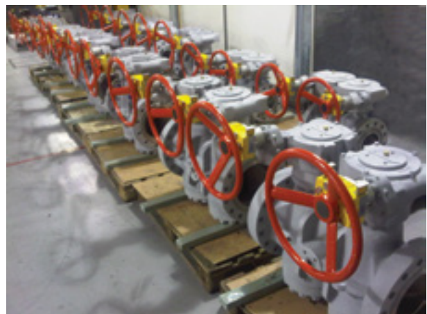
Interlock systems for valve manifolds
