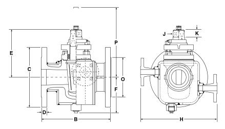
Valves have face-to-face dimensions conforming to BS 5158 PN 10/16, BS 2080 Class 150 Short, ANSI B16.10 & API 6D Class 150 Short. These valves are thus interchangeable with equivalent gate valves. Valves have Patterns conforming to BS 5353, BS 5158, API 6D & API 599 Short (with steel plug).
