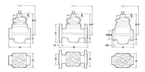
Flanged valves have face-to-face dimensions conforming to BS 5158 PN 10/16 & BS 2080 Class 150 Short, ANSI B16.10 & API 6D Class 150 Short. These valves are thus interchangeable with equivalent gate valves. Flanged valves have patterns conforming to BS 5353, BS 5158, ANSI B16.34, API 6D & API 599 Short (with steel plug).
