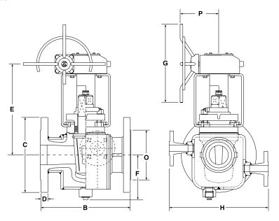
Valves have face-to-face dimensions conforming to BS EN 558 Basic Series-1.
