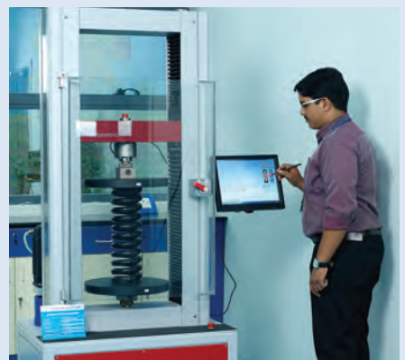
Load and deflection testing of Actuator springs
